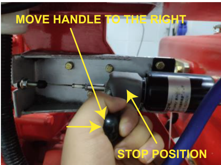
FIGURE 15 - SOLENOID RUN POSITION
