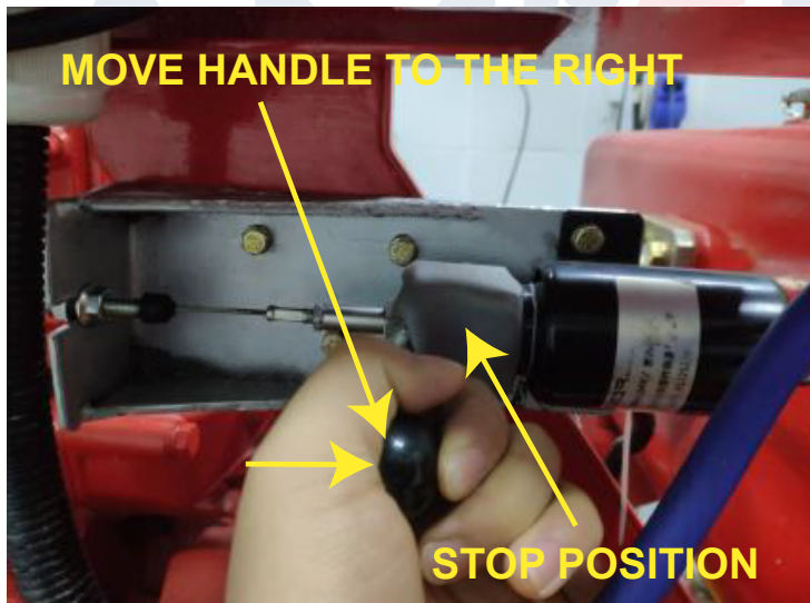
FIGURE 18 - EMERGENCY STOP USING BATTERY CONTACTORS
