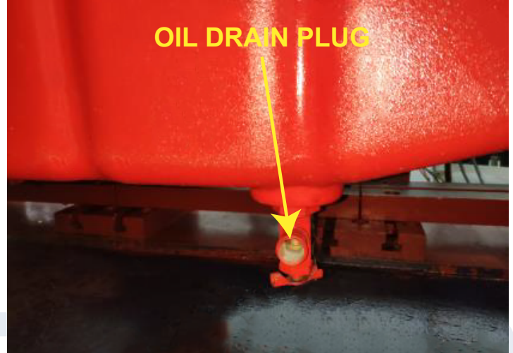
FIGURE 26 - OIL DRAIN PLUG
