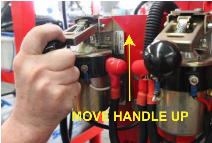
FIGURE 17 - EMERGENCY START USING BATTERY CONTACTORS
