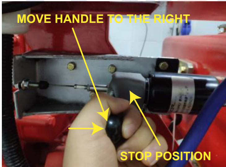
FIGURE 18 - EMERGENCY STOP USING BATTERY CONTACTORS
