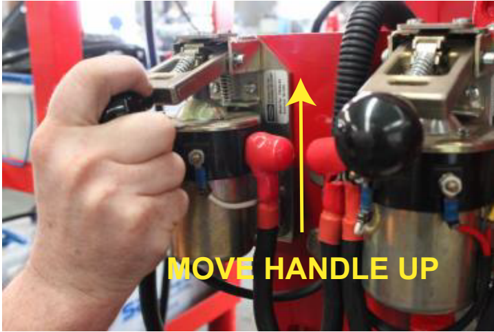
FIGURE 17 - EMERGENCY START USING BATTERY CONTACTORS
