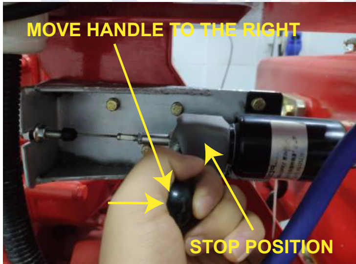
FIGURE 18 - EMERGENCY STOP USING BATTERY CONTACTORS
