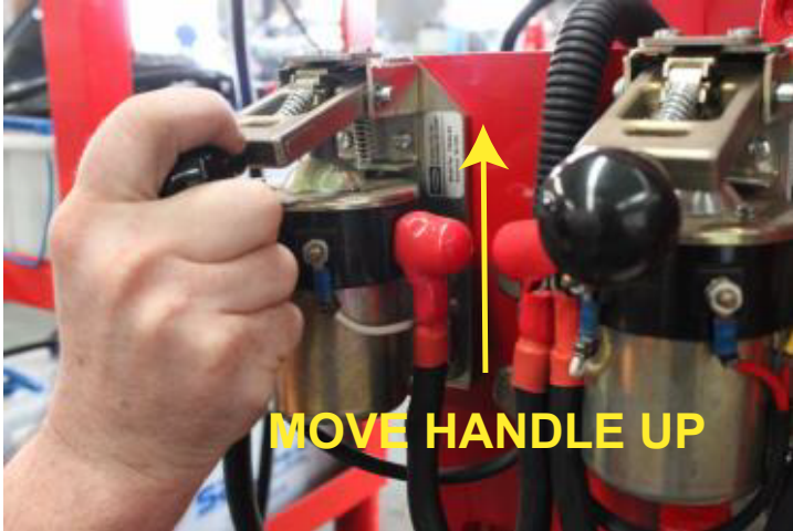
FIGURE 17 - EMERGENCY START USING BATTERY CONTACTORS
