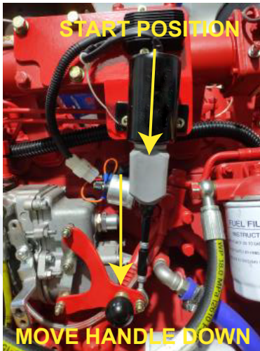
FIGURE 15 - SOLENOID RUN POSITION
