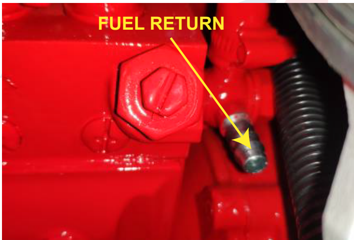
FIGURE 23 - FUEL RETURN LINE CONNECTION
