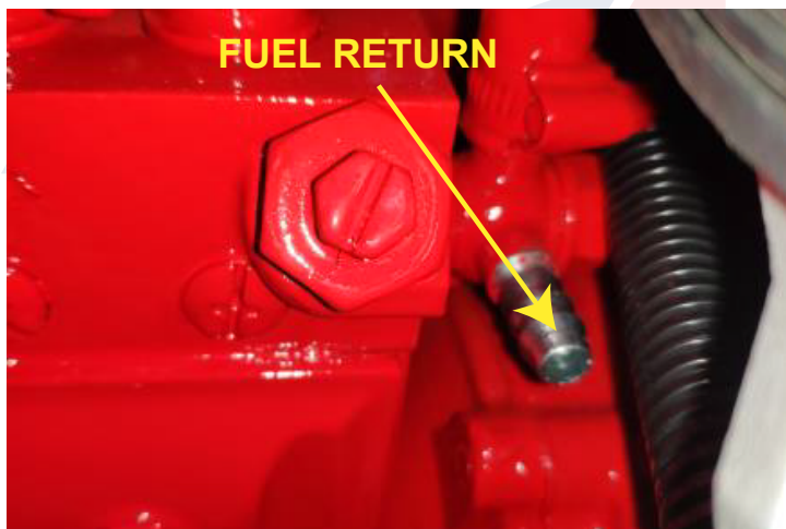
FIGURE 23 - FUEL RETURN LINE CONNECTION
