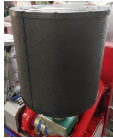
FIGURE 19 - AIR FILTER HOUSING
