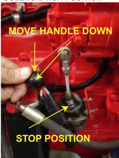
FIGURE 16 - SOLENOID STOP POSITION
