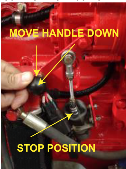
FIGURE 16 - SOLENOID STOP POSITION
