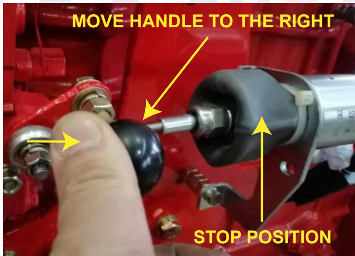
FIGURE 18 - EMERGENCY STOP USING BATTERY CONTACTORS
