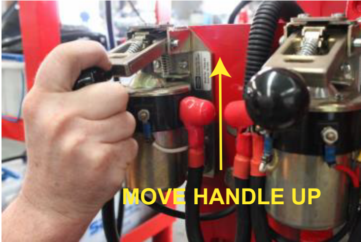
FIGURE 17 - EMERGENCY START USING BATTERY CONTACTORS
