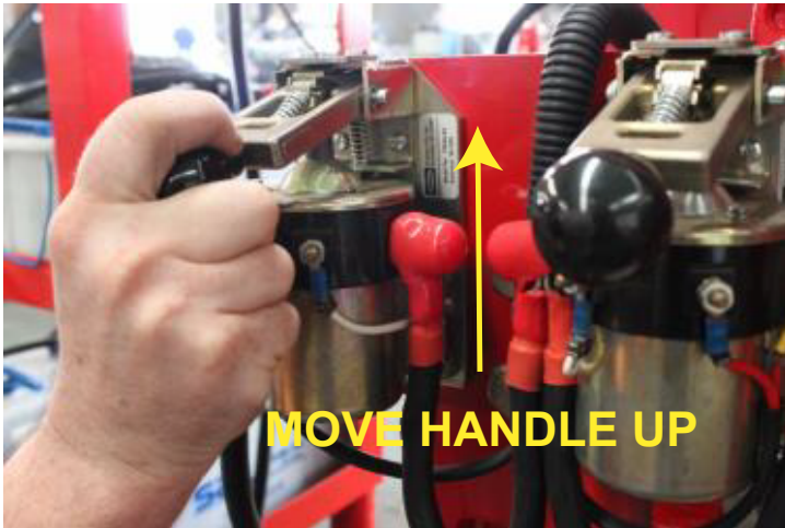
FIGURE 17 - EMERGENCY START USING BATTERY CONTACTORS
