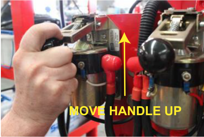
FIGURE 17 - EMERGENCY START USING BATTERY CONTACTORS
