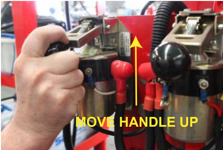
FIGURE 17 - EMERGENCY START USING BATTERY CONTACTORS
