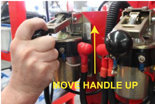
FIGURE 17 - EMERGENCY START USING BATTERY CONTACTORS
