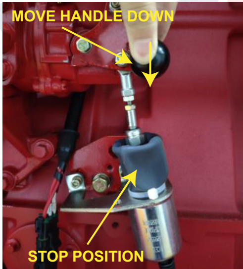
FIGURE 18 - EMERGENCY STOP USING BATTERY CONTACTORS
