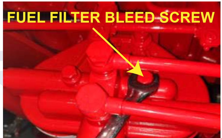
FIGURE 21 - FUEL FILTER BLEED SCREWS
