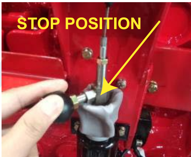
FIGURE 16 - SOLENOID STOP POSITION
