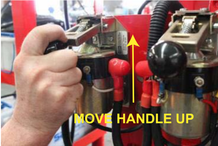
FIGURE 17 - EMERGENCY START USING BATTERY CONTACTORS
